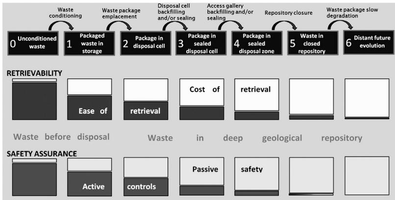
Description: A reversibility-retrievability scale defines different milestones in the execution of a final repository project (0–5), the degree of difficulty and cost level of retrieval, and the degree of active/passive safety measures. The figure is under development by the NEA and is subject to change.
