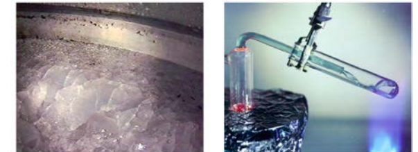
(left) Solid "Frozen" and (right) Liquid "Molten" 2LiF-BeF_2 salt
