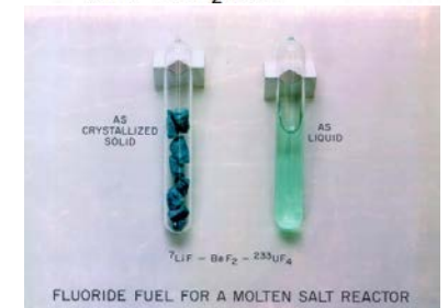
(left) Solid "Frozen" and (right) Liquid "Molten" 2LiF-BeF_2 salt
